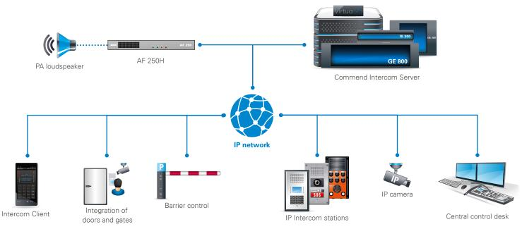
The following illustration shows an example of the integration of an AF 250H amplifier into an IP network.
