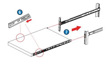
Slide the release tabs at the outer ends back on both rails.
